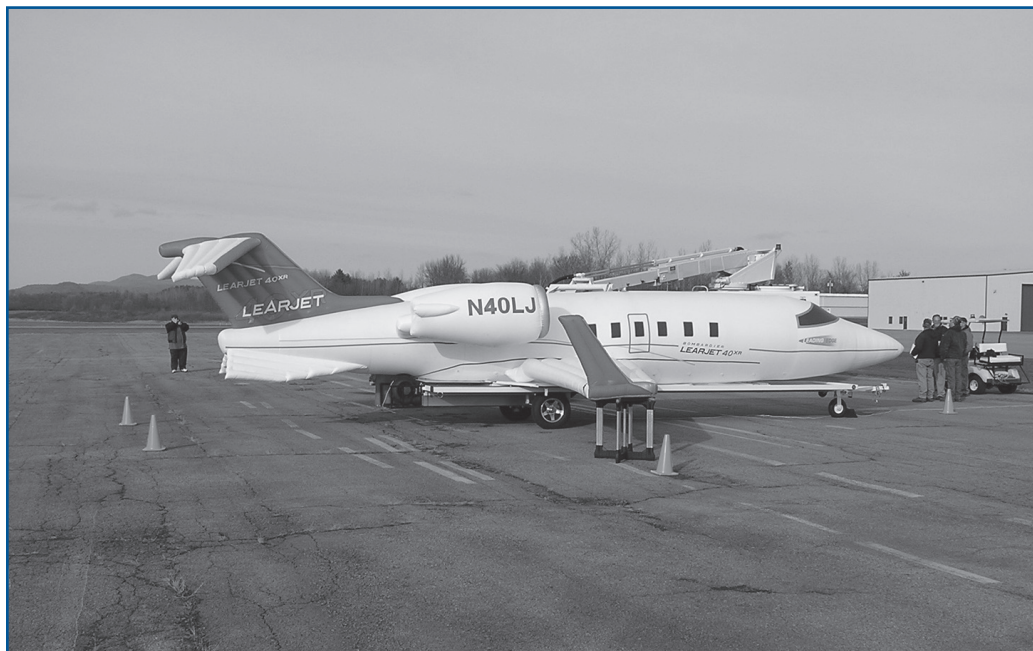
The mock-up is an inflatable simulation of a Lear 40 which is provided by Leading Edge Deicing Specialists as part of their deicing training program.
